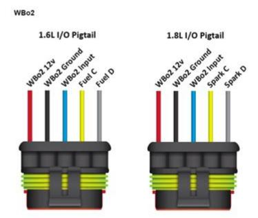
Provisions to wire your WBo2 controller are built into the ECU patch harness. Wire your pigtail to the above diagrams. An inline 5 x 20 mm 5A fuse is installed on the power wire for safety.
