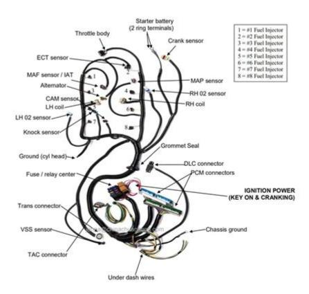
**43 vortec ignition coil wiring diagram** is a crucial component for those who are working on their Vortec engines, especially in the realm of performance upgrades or troubleshooting. Understanding the wiring diagram can help you diagnose issues quickly, improve performance, and ensure that your engine runs smoothly. This article will delve into the specifics of the 43 Vortec ignition coil wiring diagram, its components, and how to interpret it effectively.
