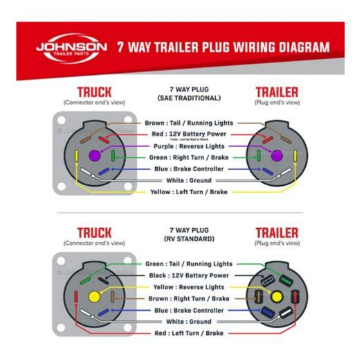
**7 way RV trailer plug wiring diagram** is a crucial topic for anyone who owns or plans to use an RV or a trailer. Understanding how to wire a 7-way RV trailer plug not only enhances safety during travel but also ensures that all features of your RV or trailer function correctly. This article will explore the wiring diagram in detail, including the purpose of each wire, common issues, and tips for proper installation.
