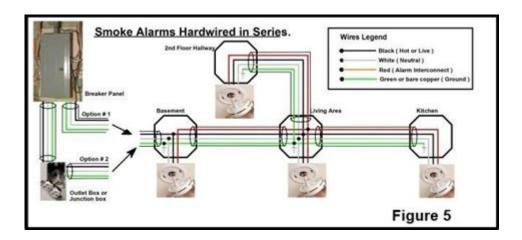
3 wire smoke detector wiring diagram is essential for anyone looking to install or replace a smoke detector in their home. Understanding the wiring configuration can not only help ensure proper functionality but also enhance safety measures in case of fire emergencies. In this comprehensive guide, we will cover everything you need to know about 3 wire smoke detector wiring diagrams, including how they work, the components involved, and step-by-step installation instructions.
