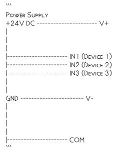
THIS DIAGRAM ILLUSTRATES HOW THE POWER SUPPLY CONNECTS TO THE MODULE AND HOW INDIVIDUAL DEVICES CONNECT TO THE INPUT TERMINALS.
