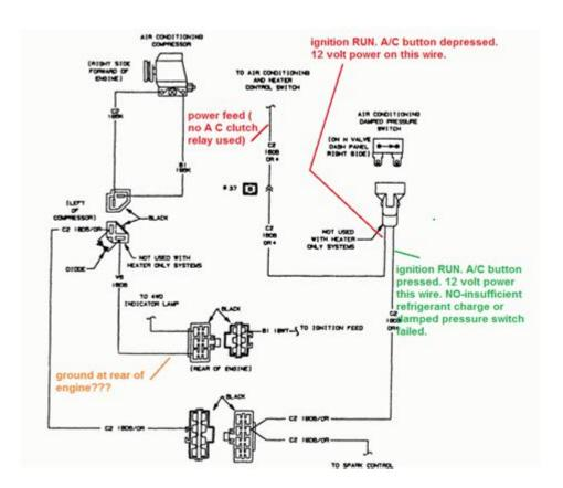
A C COMPRESSOR CLUTCH WIRING DIAGRAM IS AN ESSENTIAL COMPONENT FOR UNDERSTANDING HOW THE AIR CONDITIONING SYSTEM IN A VEHICLE OPERATES. THE A C COMPRESSOR IS RESPONSIBLE FOR CIRCULATING REFRIGERANT THROUGHOUT THE SYSTEM, AND THE CLUTCH PLAYS A CRITICAL ROLE IN ENGAGING AND DISENGAGING THE COMPRESSOR BASED ON THE VEHICLE'S COOLING NEEDS. IN THIS ARTICLE, WE WILL DELVE INTO THE IMPORTANCE OF THE A C COMPRESSOR CLUTCH, HOW ITS WIRING DIAGRAM WORKS, AND THE COMMON ISSUES THAT CAN ARISE.
