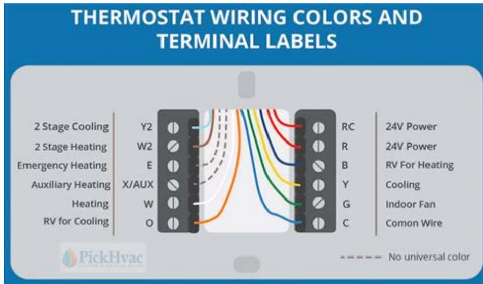
A C THERMOSTAT WIRING DIAGRAM IS AN ESSENTIAL TOOL FOR HOMEOWNERS AND HVAC TECHNICIANS ALIKE, PROVIDING A CLEAR VISUAL REPRESENTATION OF HOW TO WIRE A THERMOSTAT IN AN AIR CONDITIONING SYSTEM. UNDERSTANDING THE WIRING DIAGRAM IS CRUCIAL FOR ANYONE LOOKING TO INSTALL, REPLACE, OR TROUBLESHOOT A THERMOSTAT. IN THIS ARTICLE, WE WILL EXPLORE THE COMPONENTS OF A THERMOSTAT, THE FUNCTION OF EACH WIRE, COMMON WIRING CONFIGURATIONS, AND TIPS FOR SAFELY WORKING WITH ELECTRICAL SYSTEMS.
