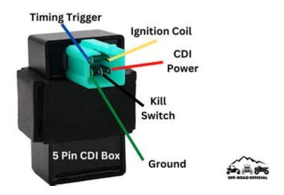
5 pin CDI box wiring diagram is a crucial element for anyone looking to understand or replace the ignition system in motorcycles, ATVs, and other small engine vehicles. A CDI, or Capacitor Discharge Ignition, system plays a vital role in controlling the ignition timing and improving engine performance. Understanding the wiring diagram is essential for proper installation, troubleshooting, and ensuring the longevity of your vehicle's ignition system.
