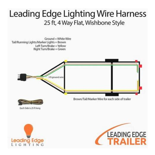
4 WAY TRAILER WIRING DIAGRAM IS ESSENTIAL FOR ANYONE LOOKING TO TOW A TRAILER SAFELY AND EFFECTIVELY.
