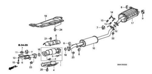
**2007 Honda CRV exhaust system diagram** serves as an essential tool for understanding the intricacies of your vehicle's exhaust system. The exhaust system plays a crucial role in reducing harmful emissions from the engine and improving overall performance. In this article, we will explore the components of the exhaust system in the 2007 Honda CRV, the importance of each part, and how to read and interpret the exhaust system diagram.
