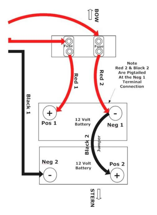
**2 battery 24 volt wiring diagram** is an essential topic for anyone looking to understand how to configure a 24-volt power system using two 12-volt batteries. This configuration is commonly used in various applications, including RVs, solar energy systems, and electric vehicles. In this article, we will delve into the specifics of wiring two 12-volt batteries to create a 24-volt system, the benefits of this setup, important considerations, and safety tips.
