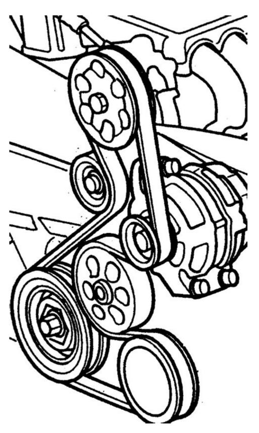
**2009 Honda Accord serpentine belt diagram** is an essential reference for any Honda Accord owner looking to service or replace their vehicle's serpentine belt. The serpentine belt is a crucial component that drives multiple accessories in the engine, such as the alternator, power steering pump, water pump, and air conditioning compressor.
