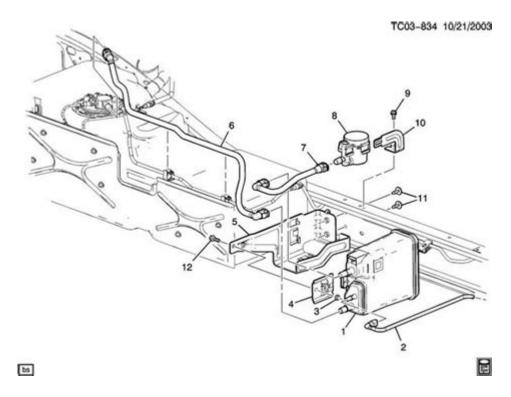
2005 Chevy Tahoe Evap System Diagram: Understanding the evaporative emissions control system in your 2005 Chevy Tahoe is crucial for ensuring your vehicle runs efficiently and remains compliant with environmental regulations. This article will delve into the specifics of the evap system, including its components, function, and maintenance tips, as well as providing a detailed diagram for better visualization.
