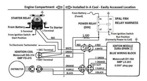
**1979 Ford ignition module wiring diagram** is a crucial resource for any DIY enthusiast or professional mechanic working on classic Ford models. Understanding the wiring diagram can simplify the troubleshooting process, enhance repair efficiency, and ensure that the ignition system operates smoothly. In this comprehensive guide, we will explore the significance of the ignition module, how to read the wiring diagram, and provide step-by-step instructions for installation and troubleshooting.
