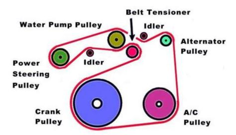
**2007 Toyota Tacoma 2.7 Serpentine Belt Diagram** is an essential reference for any Tacoma owner or mechanic working on this popular midsize pickup truck. The serpentine belt is a critical component of the engine's accessory drive system, responsible for driving multiple peripherals such as the alternator, power steering pump, air conditioning compressor, and water pump. Understanding the layout of the serpentine belt can save time and effort during maintenance or repairs.
