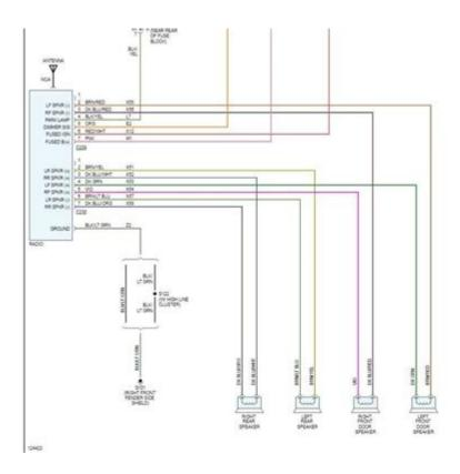
2005 Dodge Ram radio wiring diagram is an essential resource for anyone looking to install, troubleshoot, or replace the audio system in their vehicle. Understanding the wiring configuration can help ensure proper installation and functioning of the radio, which is a vital component of any driving experience. In this article, we will delve into the specifics of the wiring diagram, discuss the different components involved, and provide practical steps for using the diagram effectively.
