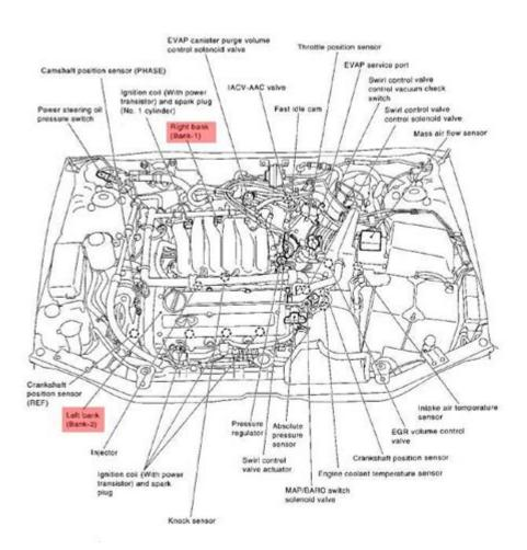
**2000 Nissan Maxima engine diagram** is an essential resource for both car enthusiasts and mechanics who wish to understand the internal workings of this popular sedan. The 2000 Nissan Maxima is equipped with a powerful V6 engine that is known for its performance and reliability. In this article, we will explore the components of the 2000 Nissan Maxima engine, provide a detailed diagram, and discuss the functions of each part to enhance your understanding of the vehicle's mechanics.
