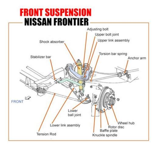
2000 Nissan Frontier front suspension diagram is an essential tool for understanding the complexities of the vehicle's front suspension system. This system plays a crucial role in ensuring a smooth ride and maintaining vehicle stability. In this article, we will explore the components of the front suspension, their functions, and how they work together, along with a detailed discussion of the 2000 Nissan Frontier front suspension diagram.
