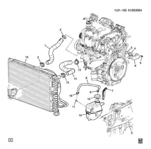
**2005 Chevy Equinox cooling system diagram** is essential for understanding how the engine's temperature is regulated and maintained within optimal operating limits. The cooling system plays a crucial role in preventing engine overheating, maintaining performance, and ensuring longevity. In this article, we will explore the components of the cooling system, how they work together, and provide a detailed diagram to enhance understanding.
