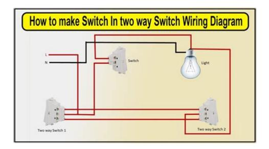
**2** way switch wiring diagram home is an essential topic for any homeowner or DIY enthusiast looking to enhance their electrical knowledge. Understanding how to wire a two-way switch correctly can empower you to control lighting from multiple locations, adding convenience and functionality to your home. This article will guide you through the fundamentals of two-way switch wiring, providing clear diagrams, steps, and safety tips to ensure a successful installation.
