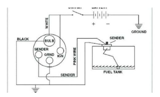
**2 wire fuel sending unit wiring diagram** is a crucial aspect for anyone working on automotive fuel systems. Understanding how to interpret and connect these diagrams ensures accurate fuel level readings and prevents potential issues in the vehicle's electrical system. In this article, we will delve into the components of a 2-wire fuel sending unit, how to read a wiring diagram, and the practical steps for installation and troubleshooting.
