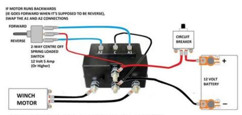
CONNECTIONS FOR 2-WIRE WINCH MOTORS
