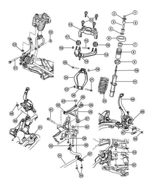
2002 Dodge Ram 1500 front suspension diagram is an essential reference for mechanics and DIY enthusiasts who wish to understand the intricacies of the vehicle's suspension system. The front suspension of the 2002 Dodge Ram 1500 plays a critical role in providing a comfortable ride, improving handling, and ensuring the safety of the vehicle. In this article, we will explore the components of the front suspension system, their functions, and how to interpret the diagram effectively.
