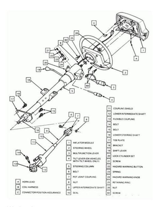
2005 CHEVY SILVERADO STEERING COLUMN DIAGRAM IS A VITAL RESOURCE FOR ANYONE LOOKING TO UNDERSTAND THE INNER WORKINGS OF THIS POPULAR PICKUP TRUCK. THE STEERING COLUMN PLAYS AN ESSENTIAL ROLE IN VEHICLE CONTROL AND SAFETY, AND HAVING A DETAILED DIAGRAM CAN SIGNIFICANTLY AID MECHANICS AND DIY ENTHUSIASTS IN TROUBLESHOOTING, REPAIRS, AND MODIFICATIONS. IN THIS ARTICLE, WE WILL EXPLORE THE ANATOMY OF THE STEERING COLUMN, ITS FUNCTIONS, COMMON ISSUES, AND HOW TO UTILIZE THE DIAGRAM EFFECTIVELY.
