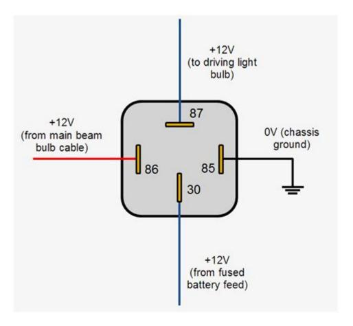
12v relay wiring diagram 4 pin relays are essential components in many electrical systems, providing a means to control high-power devices with low-power signals. Understanding how to wire a 4-pin relay properly is crucial for ensuring safety and functionality in your projects. In this article, we will delve into the components of a 12V relay, explain how a 4-pin relay works, and provide detailed wiring diagrams and applications.
