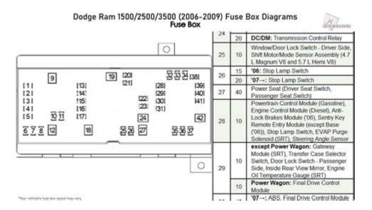
**2006 Dodge Ram fuse box diagram** is an essential tool for any Dodge Ram owner or mechanic. Understanding the layout of the fuse box can help diagnose issues related to electrical systems, ensuring that both the vehicle and its components remain in optimal working condition. This article will explore the layout of the fuse box in the 2006 Dodge Ram, describe the function of various fuses, and provide troubleshooting tips for common electrical problems.
