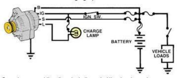
Four wires connect the alternator to the rest of the charging system. 'B' is the alternator output wire that supplies current to the battery. 'IG' is the ignition input that turns on the alternator/regulator assembly. 'S' is used by the regulator to monitor charging voltage at the battery. 'L' is the wire the regulator uses to ground the charge warning lamp.
